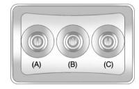
The A/V jacks, located on the rear of the floor console, allow audio or video signals to be connected from an auxiliary device such as a camcorder or a video game unit to the RSE system. Adapter connectors or cables (not supplied) might be required to connect the
